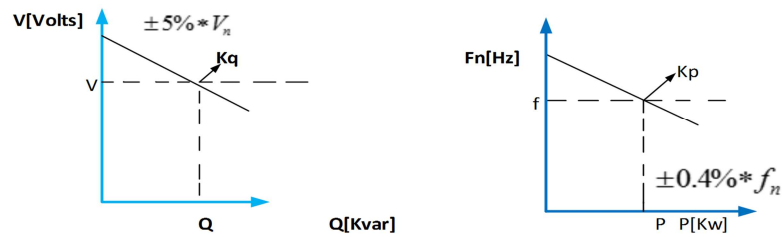
Figure 3. Schematic diagram of droop control.
