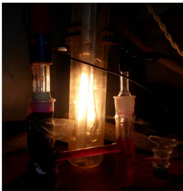
Figure 2. Set-up of photogalvanic cell.
