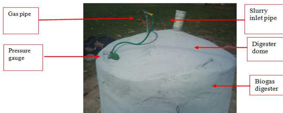
Figure 2. The constructed biogas digester with no insulation.
